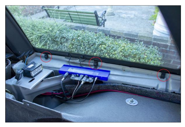
4. Set the panel to one side - you should now be able to see the receiver on top of a metal framework, it is the small black box nearest the rear seats.
