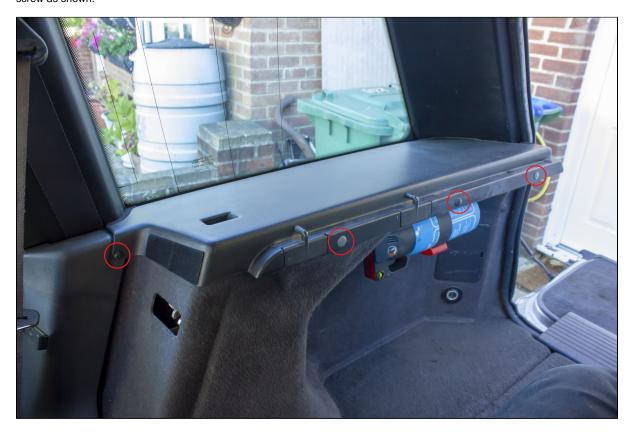
3. Lift the panel starting from the rear seat end. It will need to be levered upwards with moderate force - there are three metal clips along the window edge that the panel should release itself from.
