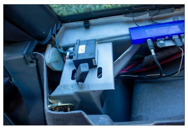
5. Position the Fob Filter unit on the inside of the supporting diagonal metalwork, and secure it in place with a cable tie.
