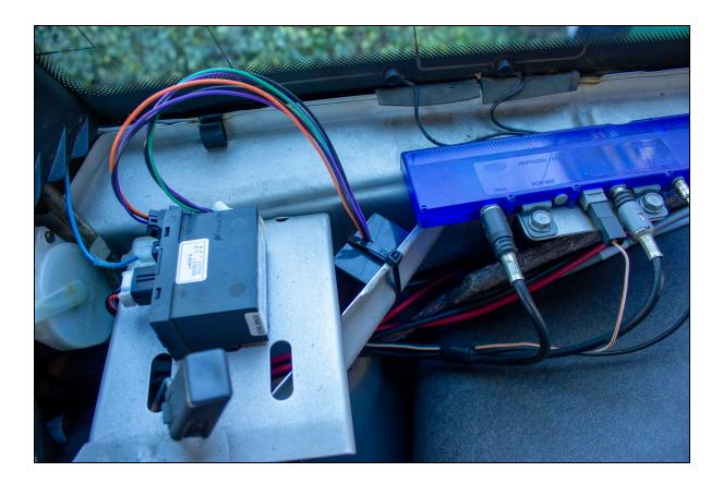
6. Unplug the white three pin connector from the receiver by depressing the tab and pulling the connector body - do not pull on the wires! A flat bladed screwdriver or similar implement may be used to help lever the plug out from the receiver while depressing the tab - they can be somewhat stiff. Connect this into the black socket on the filter unit, and connect its own white plug back into the original receiver.
